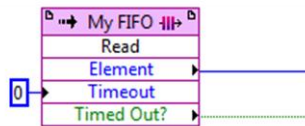
Figure 89. FIFO Read operations inside the SCTL must use a timeout of zero. The Time Out? output indicates an empty FIFO.
