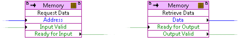
Figure 93. DRAM reads are performed by requesting data from a given address and then retrieving it some cycles later when the Output Valid signal of the Retrieve Data method is TRUE .
