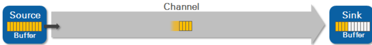
Figure 85. Buffering helps handle transient conditions by temporarily storing data on the source or sink.
