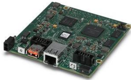
Figure 8. NI Single-Board RIO takes the embedded RIO platform to smaller form factors and deployment applications.
