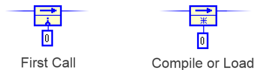
Figure 75. With Feedback Nodes set to initialize on Compile or Load , you use fewer resources and can compile at higher rates.
