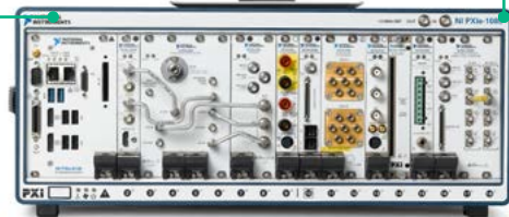
FIG 2 PXI is a rugged PC-based platform for measurement and automation systems.
