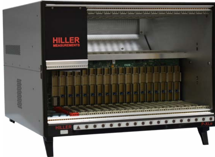
FIG 6 | The P-XLe chassis was developed to accommodate measurement science that cannot be managed in the Eurocard PXI format. It is ideally suited for the commercially obsolete VXI standard. (Image courtesy of Hiller Measurements.)
