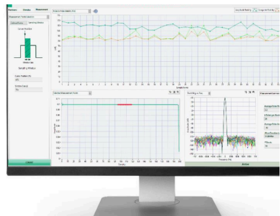
FIGURE 07 Measurement Panel for Taking Pulse Profile and Stability Measurements Included with the Pulsed RF Measurements Library
