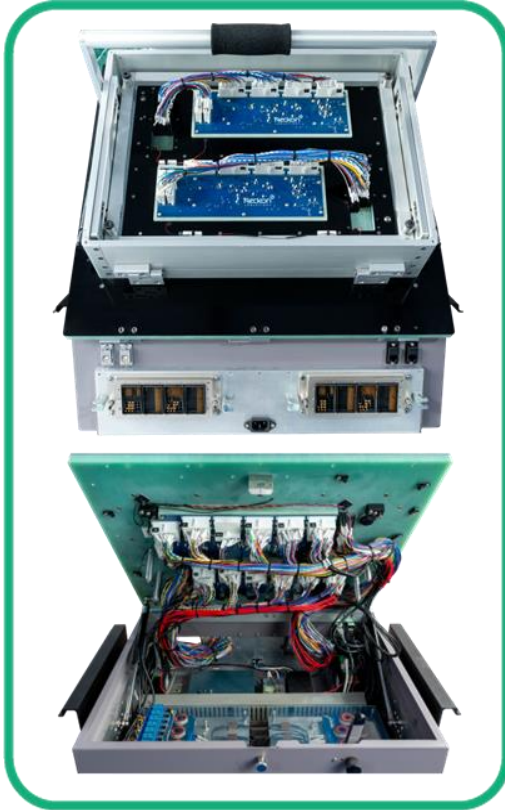
Fixture Wireless PCBA interface - Mirror signal contacts
