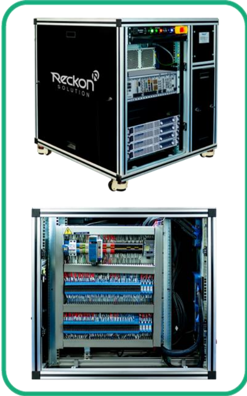
Test Rack PXI Technology
