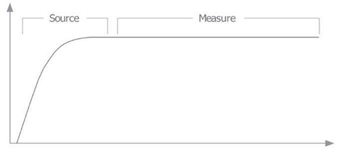
FIGURE 4 Illustration of the Aperture Time of an SMU with Respect to a Sample Signal
