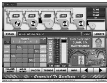
connected the new Lookout computer system to the existing SCADA system with a high-speed communications link.
