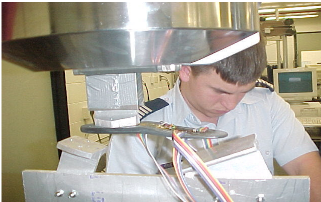
Figure 1. Strain gage testing of the Springlite prosthetic foot.
